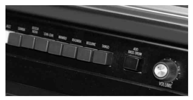
FIGURE 6.13 Detail of an analog Hammond Rhythm II unit, a part of a Hammond T-422 organ manufactured in 1969. This unit allows two dance rhythms to be superimposed on top of each other with a variable tempo control.
