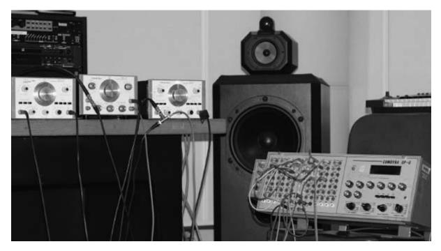
FIGURE 10.1 Setup for Xopher Davidson and Zbigniev Karkowski's album *Processor* (2010). The Wavetek waveform generators (left) are controlled by a Comdyna GP6 analog computer (right). Photograph by Curtis Roads in Studio Varèse at UCSB.
