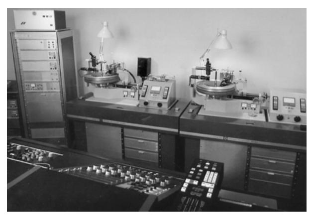
FIGURE 12.10 Analog mastering studio with two disc-cutting lathes. Notice the black microscopes above each turntable.
