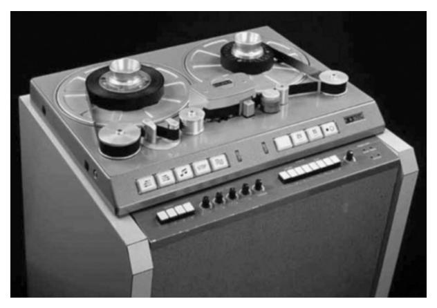
FIGURE 12.2 Studer J37 four-track tape recorder, introduced in 1964. This model was used to make the Sgt. Pepper's Lonely Hearts Club Band album by The Beatles, a tour-de-force of multitrack recording and mixing.
