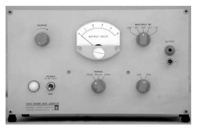
FIGURE 4.19 General Radio analog noise generator.
