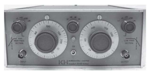
FIGURE 4.15 Krohn-Hite 3550 analog filter.
