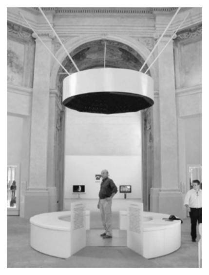
FIGURE 8.21 Acoustic chandelier, La Casa della Musica, Parma, Italy. The chandelier contains 224 loudspeakers for wave field synthesis.
