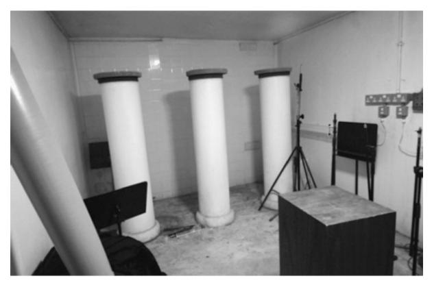
FIGURE 8.1 Echo chamber at Abbey Road Studios with tiled wall and pillars to enhance sound reflection.
