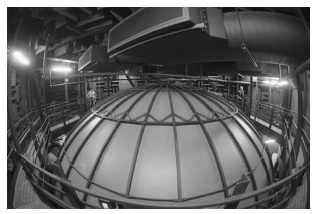
FIGURE 8.22 The UCSB AlloSphere viewed from outside. The AlloSphere is a three-story-high laboratory instrument for 3D immersive visual and audio projection with a multichannel Meyer Sound system (Amatriain et al. 2007, 2008, 2009). Photograph by Paul Wellman.
